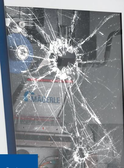
**Protected thanks to polycarbonate windows**: The polycarbonate windows on your MÄGERLE surface and profile grinding machine protect the machine operator from the fragments of a shattered grinding wheel in the event of a machine crash.
