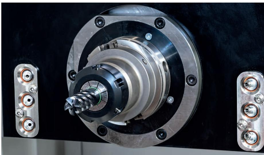
Nozzles are available on the grinding support for drilling and milling tools, and a coolant supply can be optionally provided through the spindle.
