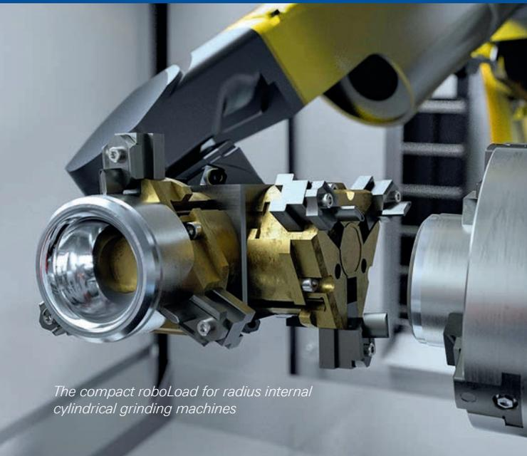
The compact roboLoad for radius internal cylindrical grinding machines
